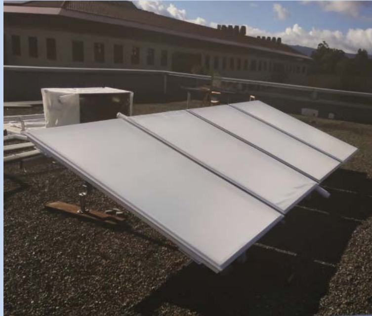
Fig. T6-2: Radiative cooling panels operable during the day 53
