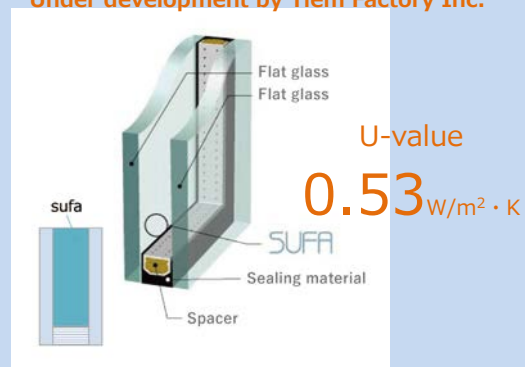
Fig. T5-3 Estimated performance of hybrid aerogel window 50
