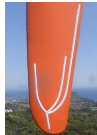
Diverter strips applied in a field
