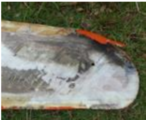
Blade failure by lightning
